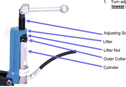
1. Turn adjusting screw until outer collar is at it's lowest limit of travel. Do this for EACH cut.
